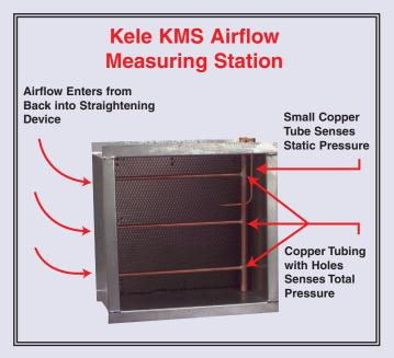
Now that both static pressure and total pressure can be sensed, a differential pressure transmitter, such as the **T30**, **M264**, or the high accuracy **XLdp** is used to measure velocity pressure. Selecting the scale for a differential pressure transducer for an airflow measuring station can be done using the following equation:
