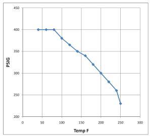
\*Max. Temp. 260° F (126.7° C) 230 psig Unit can be used to 20° F ( $-6.7^{\circ}$  C) @ 400 psig
