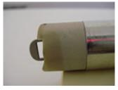
Installation is now complete. If done properly, when spun by hand, the impeller will spin freely on the shaft, and glide smoothly to a stop.
