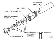
Fig. 4. Capillary compression fitting.
