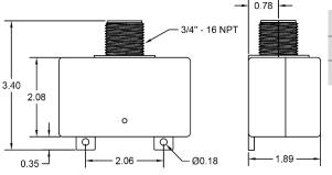
**DITEK's DTK-HW Series** of surge protective devices are designed and manufactured to meet the standards of the life safety industry. These compact, parallel-mount SPD's are available for 120V, 240V and 120/240V systems; and are widely used to protect fire alarm panels and other dedicated branch circuit loads. Their small footprint enables installation in a variety of locations.
