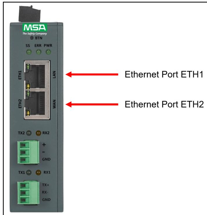
The Ethernet Port is used both for Ethernet protocol communications and for configuring the gateway via the Web App. To connect the gateway, either connect the PC to the router's Ethernet port or connect the router and PC to an Ethernet switch. Use Cat-5 cables for the connection.
