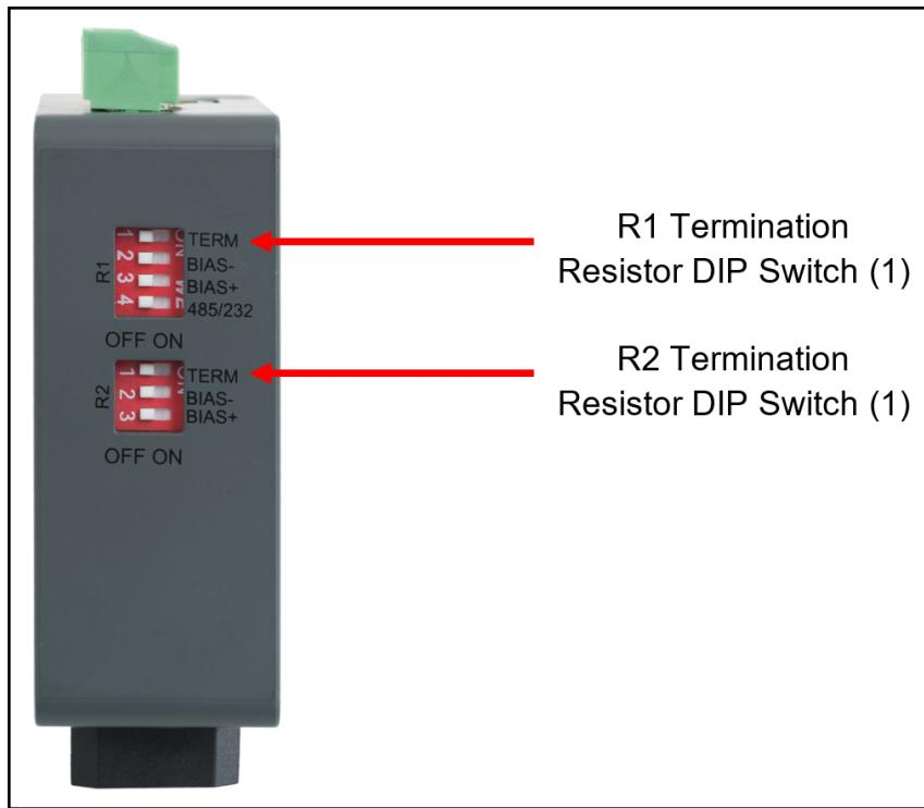
If the gateway is the last device on the serial trunk, then the End-Of-Line Termination Switch needs to be enabled. **To enable the Termination Resistor, move the TERM dip switch to the right in the orientation shown in above.**
