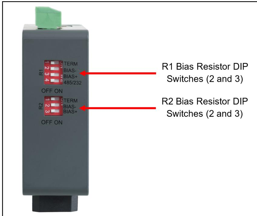
To enable Bias Resistors, move both the BIAS- and BIAS+ dip switches to the right in the orientation shown above.
