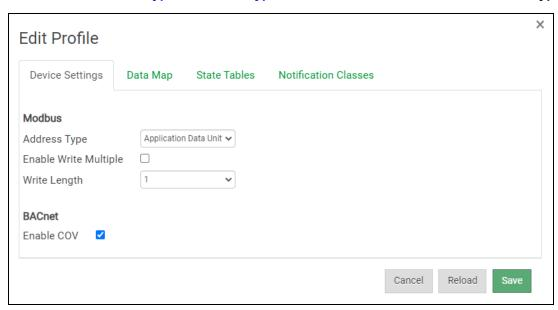
If using a BACnet State Table, click on the "State Table" tab to define the table and its variables.
