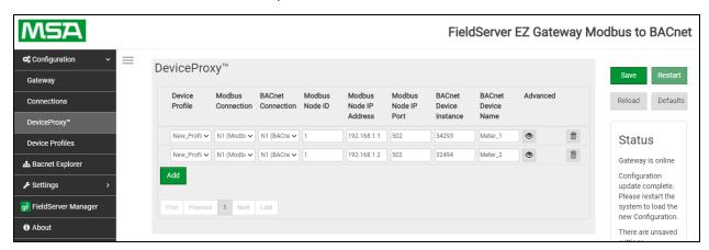
NOTE: If required, click the Advanced Settings button (eye icon) to enter the Device Description and Device Location.
