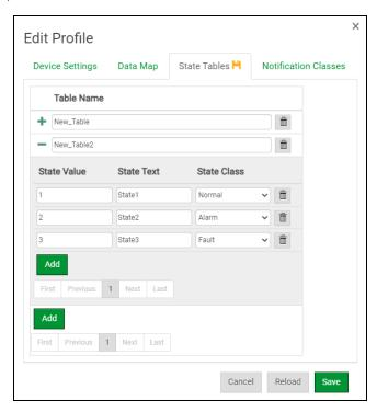
NOTE: The Table Name field must be 14 characters or less. No commas allowed. The State Text field must be 50 characters or less. No commas allowed.
