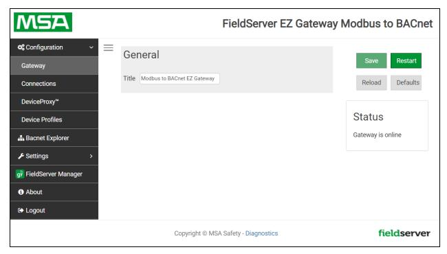
NOTE: The FieldServer Manager tab FieldServer Manager (see screenshot above) allows users to connect to the Grid, MSA Safety's device cloud solution for IIoT. The FieldServer Manager enables secure remote connection to field devices through a FieldServer and its local applications for configuration, management, maintenance. For more information about the FieldServer Manager, refer to the MSA Grid - FieldServer Manager Start-up Guide.
