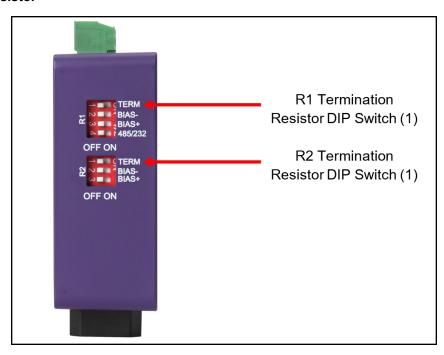
If the gateway is the last device on the serial trunk, then the End-Of-Line Termination Switch needs to be enabled. **To** enable the Termination Resistor, move the TERM dip switch to the right in the orientation shown in above.
