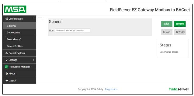
NOTE: For BACnet/IP, click on the Connections tab to ensure the gateway is on the BACnet/IP network subnet to configure BBMD.
