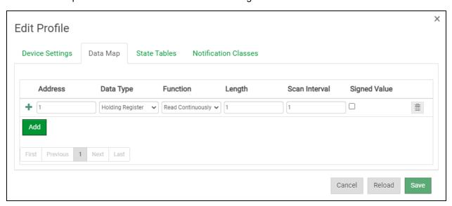
NOTE: Check the Signed Value checkbox (right of the data map entry) if signed values are needed.
