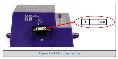
The following Baud Rates are supported on the R1 Port:
