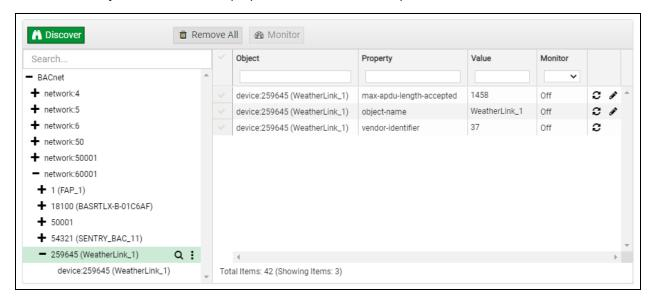
• To view the full details of a device, highlight the device directly (in the image below – "1991 WeatherLink\_1") and click the Explore button ( ) that appears to the right of the highlighted device as a magnifying glass icon or double-click the highlighted device.
