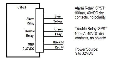
Note: There is a jumper on the PCA to change the alarm output. Remove the jumper for N.C. or leave the jumper in place for N.O.
