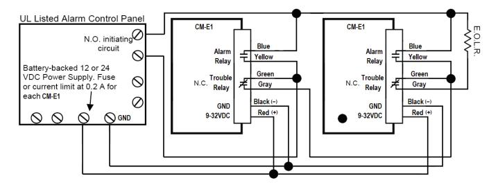
The relay of the CM-E1 is a dry contact and rated at 100mA, 40VDC. It is **not suitable for fan control** use. When connecting the units to remote buzzers or other devices (all buzzers or "other devices" must be UL approved), make sure that the load does not exceed the relay's rating. External buzzers must be capable of generating a sound output greater than 85 dBA at 10 ft (3.048 M).
