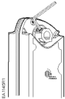
Figure 5. Fasten the Shaft Adapter to the Damper Shaft.
