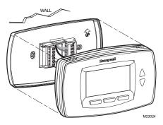
Fig. 24. Mount thermostat to wallplate.
