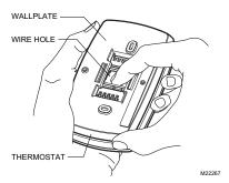
Fig. 2. Separate wallplate from thermostat.
