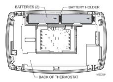
Fig. 22. Installing batteries.
