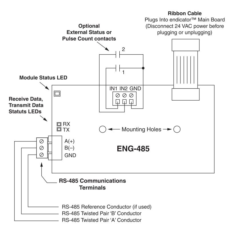
RS-485 twisted pair is polarity sensitive.
