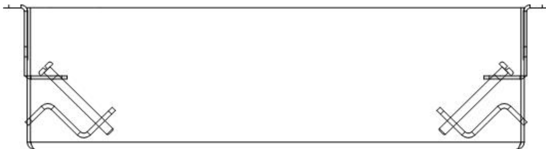
Figure 8: Retrofit Clamps Pivoted Inward
