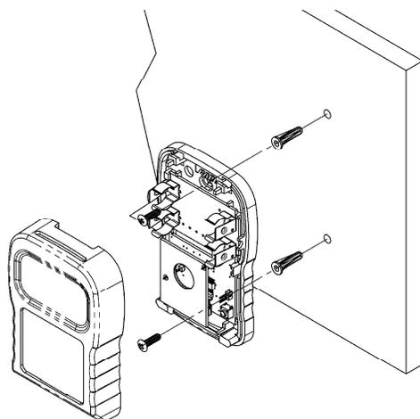
Figure 2: Drywall Mounting
