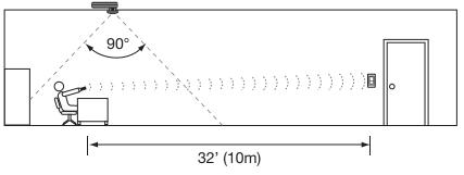
The LMRH-101 operates DLM lighting loads by transmitting IR signals to any DLM IR-enabled device within line of sight in a range of approximately 32 feet (10 meters).
