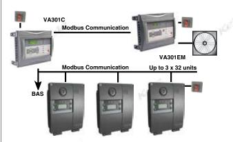
Supports Modbus protocol to daisy-chain detectors, providing up to 96 points of monitoring on a serial bus. Excellent option for controllerbased (VA301C) installations common in larger applications. A relay output is provided as an option for activating ventilation directly (e.g. when fan is located in close proximity to detector).
