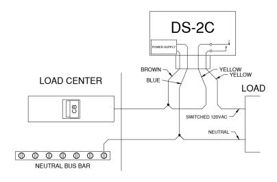
120VAC In, 120VAC Load, Heat Cable or Similar (Also Applies To 277VAC)
