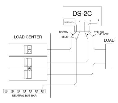
120VAC In, 240VAC Load, Separate Feed
