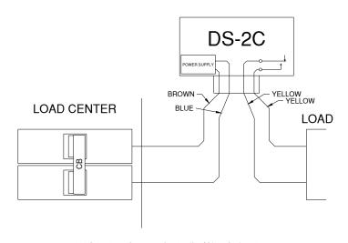
240VAC In, Dry Contact for Boiler/Circulation Pump
