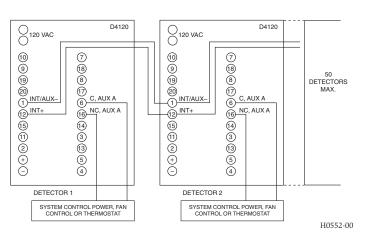
Figure 7. Multiple Fan Shutdown (interconnection of D4120 to DH100ACDC):
