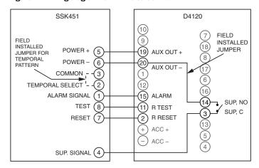
NOTE: WIRING DIAGRAM SHOWN IS FOR D4120 4-WIRE DUCT SMOKE DETECTOR SYSTEM EQUIPPED WITHOUT A CONTROL PANEL.
