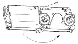
REMOVE SCREW AND PIVOT DETECTOR AS SHOWN ABOVE.
