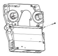
REPLACE SCREW TO SECURE DETECTOR IN PLACE.
