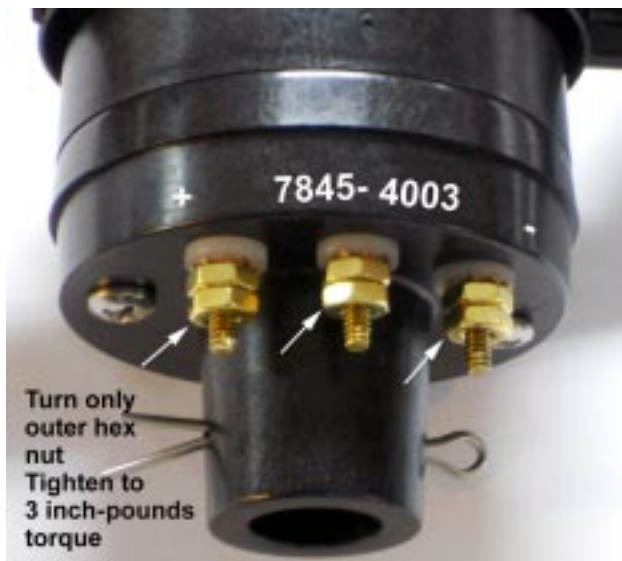
Figure 4 Wind Vane Terminals
