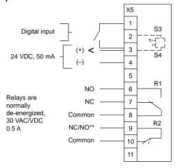
S3 = Built-in horn S4 = Switched output
