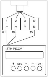
**TF, LF, AFRX Series**Connect to the installed wires of the actuator.
